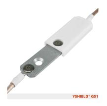
Small and flat grounding plate 20x80 mm for installation directly on top of shielding products and grounding straps. For the skirting board area. Installation preferably in the baseboard area (due to its small grounding surface) with shielding paint, shielding mesh. Usage only on the interior. One piece per wall is necessary due to the small contact area. Height when completely mounted is only 4 mm (without cover) or 6 mm (including cover).
