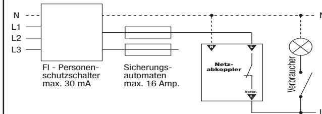
Switch off the Main Switch for the electricity supply before installation. Connect input "N" with the neutral conductor bar and input "L" with the output of the desired circuit breaker. Switch on the main switch.
